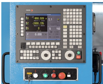
Compact control unit with electronic hand-wheels
