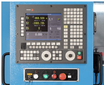
Compact control unit with electronic hand-wheels
