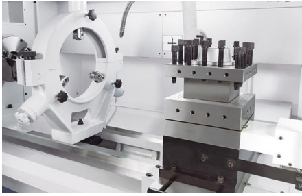
Automatic changing 4-fold steel holder
