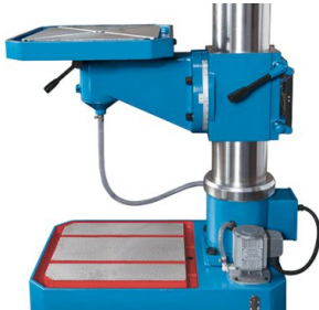
Drill press table with motorized travel and adjustable angle
