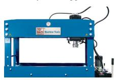
The hydraulic cylinder can be moved laterally and is clamped mechanically
