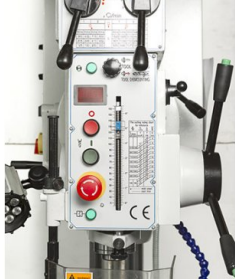
Rpm adjustment via manual transmission, and spindle rotation reversal via limit switch at depth stop
