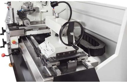
Servo drive technology – including "teach-in" Buttons that allow setting a limit stop at the current position
