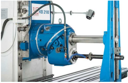
Rigid outer arbor system for long milling arbors
