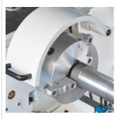
Chuck guard with integrated intelock system
