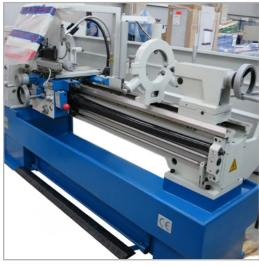
A heavy ribbed machine bed and a massive onepiece cast-iron frame provide the solid basis for this machine
