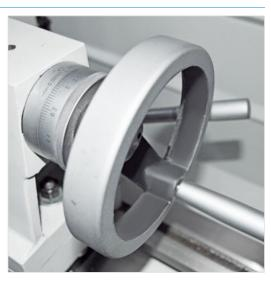
The quill can be positioned with ease using a handwheel with precision scale
