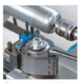
This model is equipped as standard with high quality German type quick change tool post to easily switch the tools with repeat accuracy of 0,0004 in
