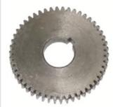
Change gears for thread cutting
