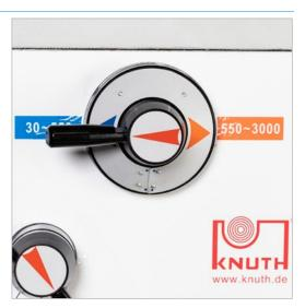
The frequency inverter reduces the number of speeds to only two, with infinitely variable speed adjustment
