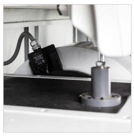
Additionally, a spindle cover is provided to protect the operator. It integrates an interlock system, stopping the spindle when to cover is lifted
