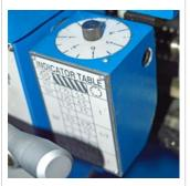
Facilitates the thread cutting process.
