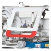
Large cover to protect the operator against chips and coolant splashes
