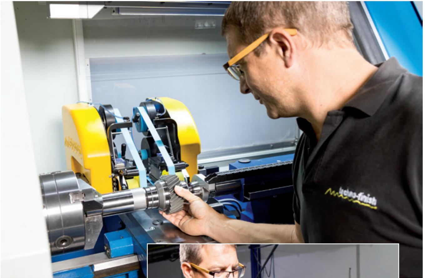
Control of reliable workpiece clamping, visual inspection of the workpiece surfaces
