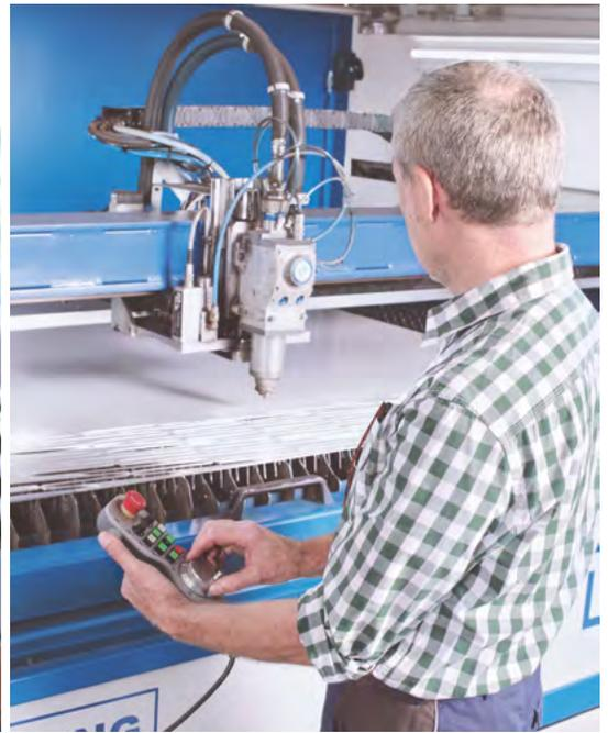
The conversion from a conventional die-cutting operation to laser technology has paid off: Now, Rauh can go from drawing to finished workpiece on the same day.
