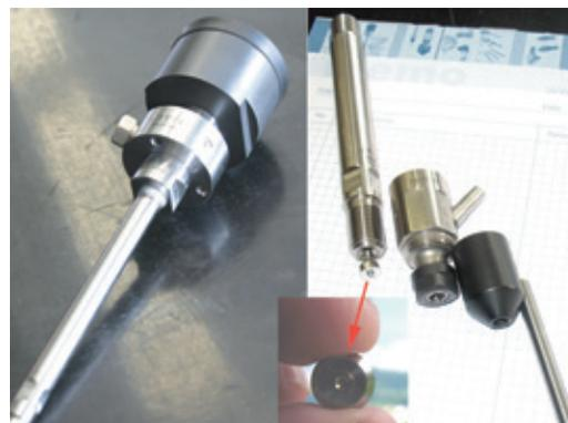
The cutter head of the water-jet cutting system handles pressures up to 4000 bar. In the center of the image: holder with hair-fine nozzle that forms the water-jet (photo: Klaus Vollrath)
