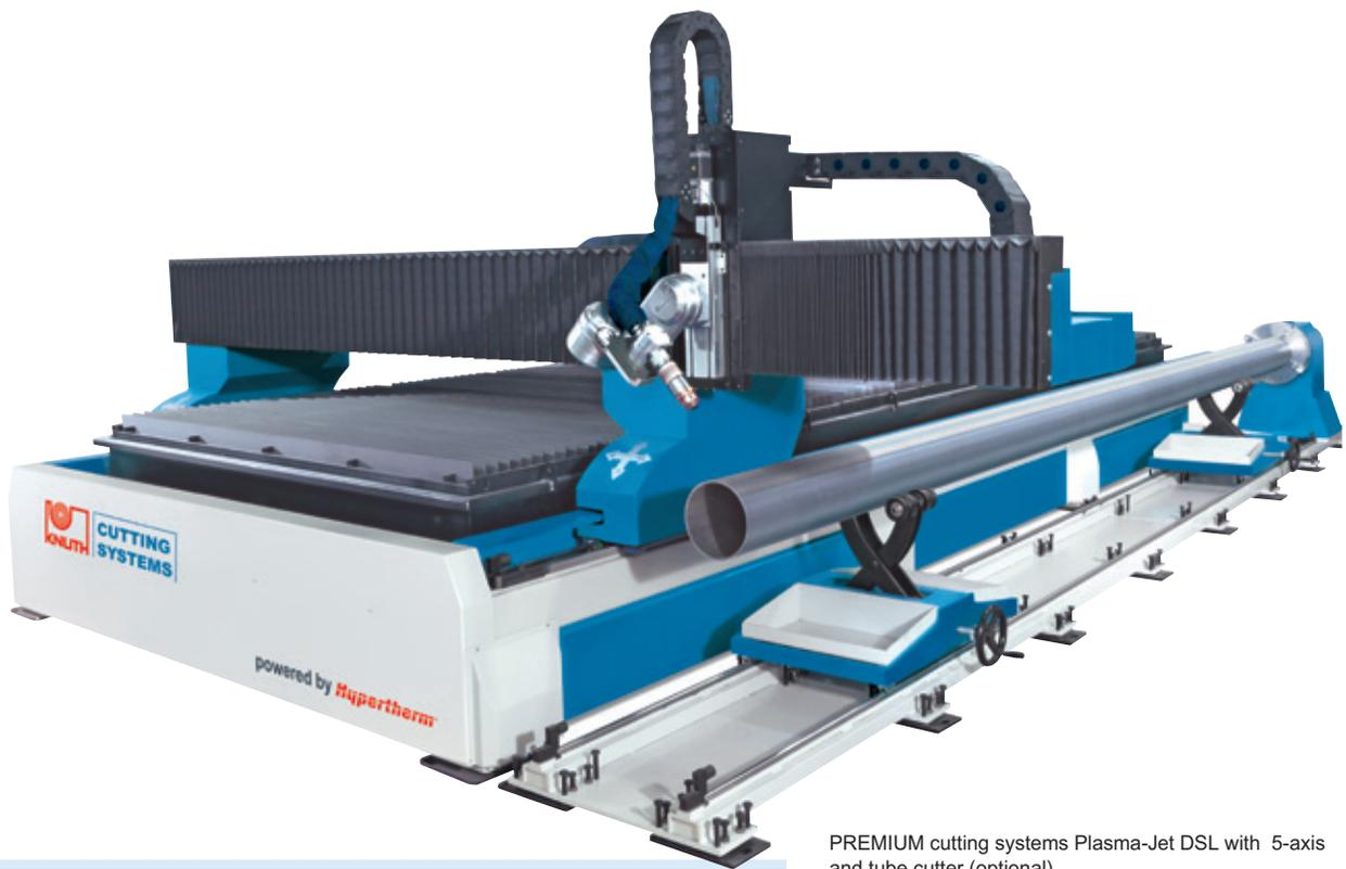
PREMIUM cutting systems Plasma-Jet DSL with 5-axis and tube cutter (optional)
