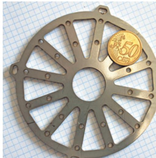
Component cut from a 2 mm thick stainless steel plate using a laser cutter (photo: Klaus Vollrath)
