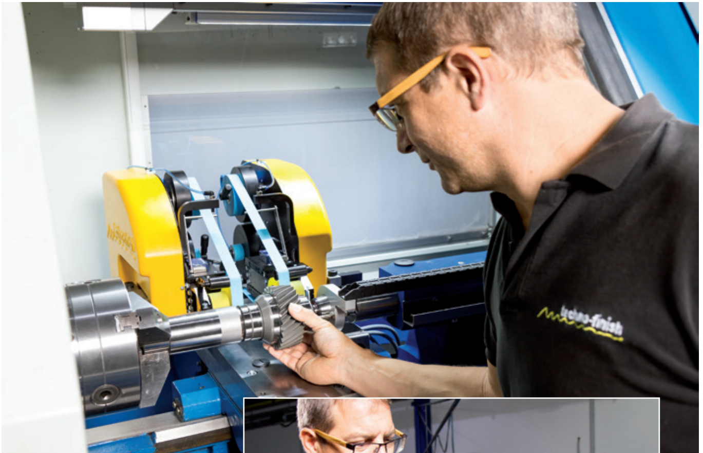
Control of reliable workpiece clamping, visual inspection of the workpiece surfaces
