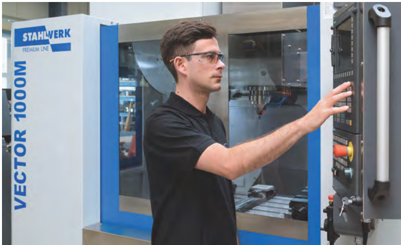
Siemens 828D Shopmill user interface ensures easy operation
