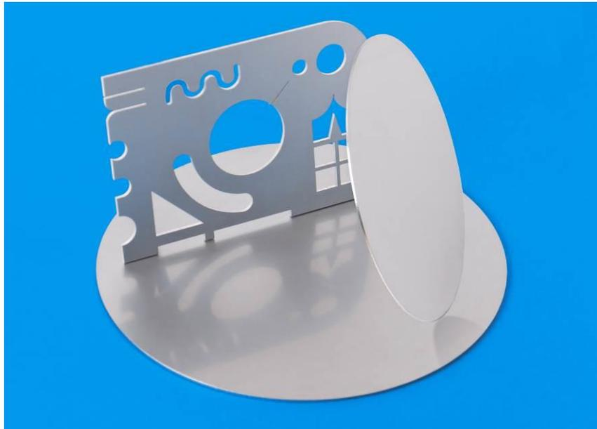
Stainless steels can be cut by the 2 kW fiber laser up to a thickness of 6 mm with a very high cut quality. Here, since nitrogen is used as the cutting gas, the cut surfaces are smooth and bare metal, as well
