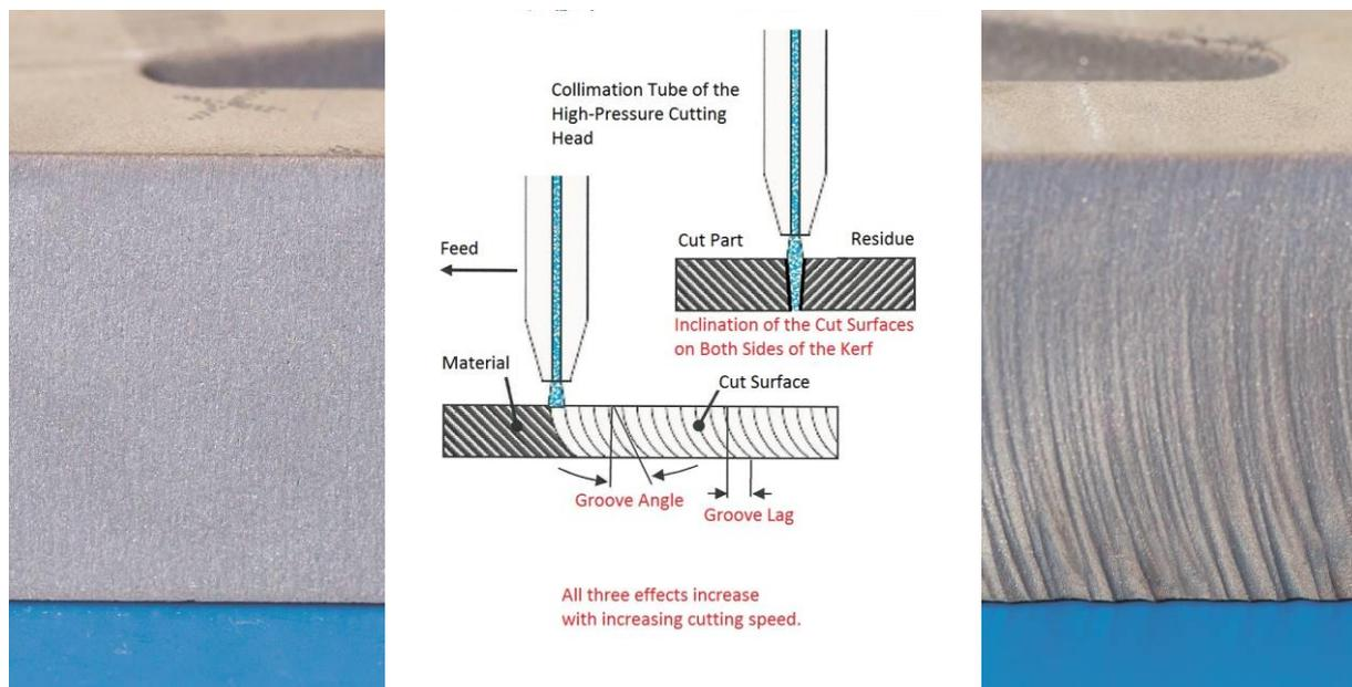
Figure 2 Cutting surfaces on 25mm thick plates of stainless steel
