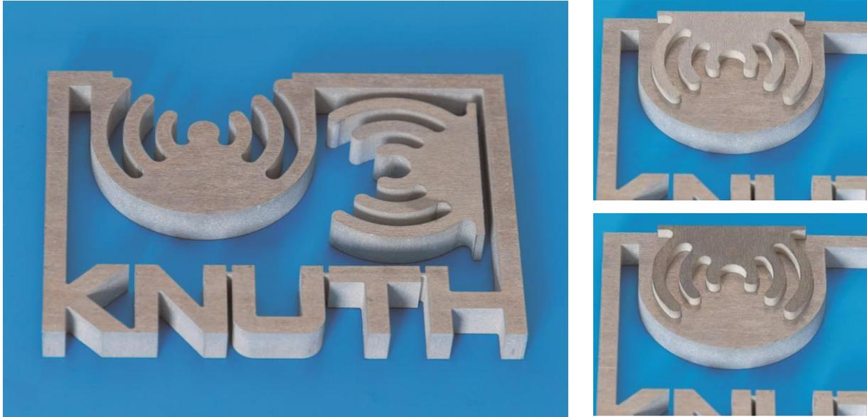
Figure 4 Waterjet-produced cut pattern (two pieces) made from 10mm thick aluminum sheet. The back plate side has been stained before (appears darker).
