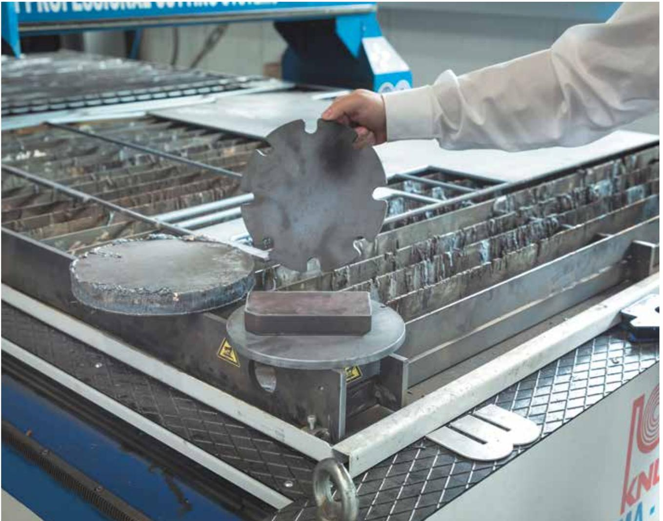
A leap forward in respect to quality: The left component has been cut with a manual plasma cutter prior to this purchase. The center part with precision cut edges was cut with the KNUTH Plasma-Jet.
