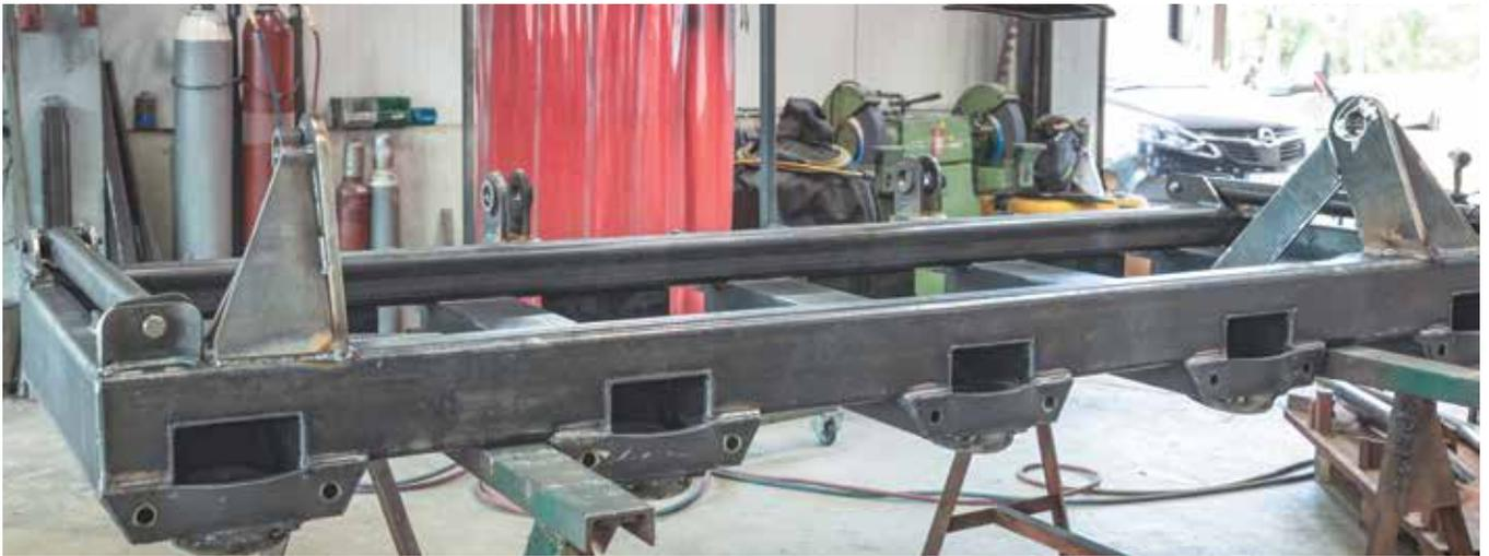
One finished part welded from a variety of cut parts that were produced with a KNUTH Plasma-Jet
