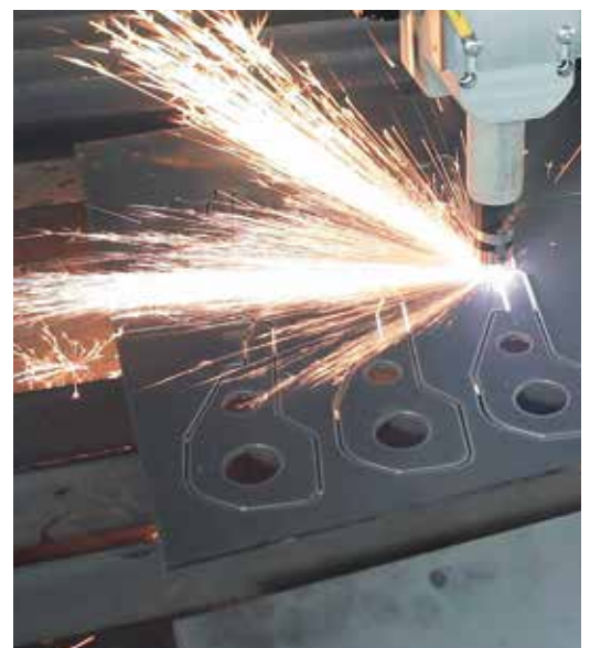
A leap forward in respect to quality: The left component has been cut with a manual plasma cutter prior to this purchase. The center part with precision cut edges was cut with the KNUTH Plasma-Jet.
