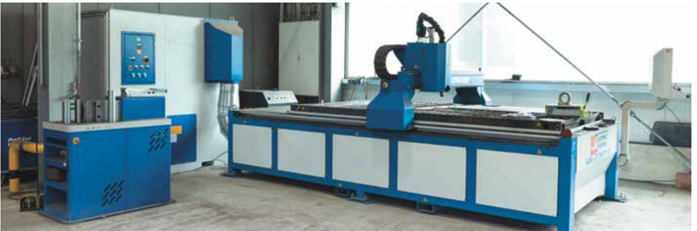
The KNUTH Plasma-Jet Compact 1530 with MaxPro 200 plasma source and vacuum exhaust system
