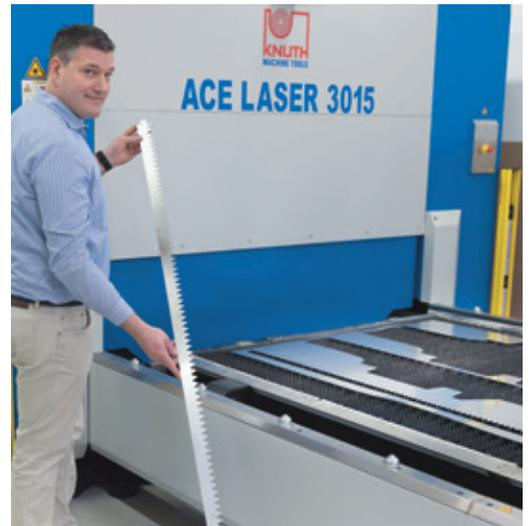
An automatic changer table system minimizes down-times.
